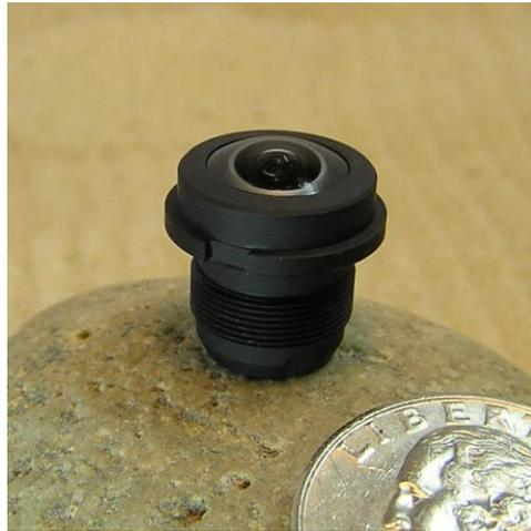
The DSL216 also features a small form factor of about 16mm maximum diameter and a total track of about 18mm. The lens barrel is threaded M12x0.5 (s-mount) to fit most standard, board-level mounts. The standard lens is provided with an integrated IR cut-off coating. For near-IR applications, lenses without the IR cut-off coating are also available.
